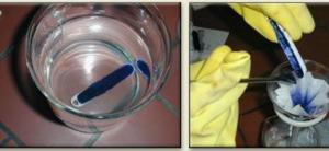
The still hot glassy product is being pulverised by immersion into cold water
