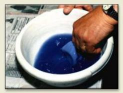
The fine particles are mixed with alcohol and poured over magnetized channel to remove the magnetic pyrite particles
