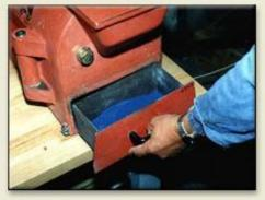
The mineral is first ground in an electric mill
