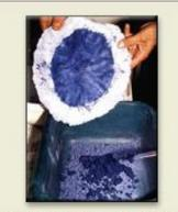
The resulting mass is kneaded with wax and water and pressed through fine cloth. The less valuable coarse "ultramarine ash" stays in the cloth
