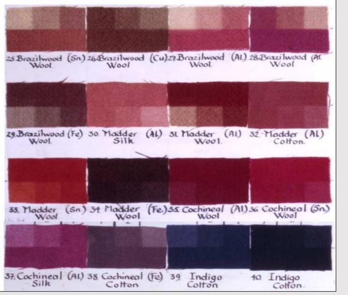
Light fastness tests of textiles dyed with natural colorants. Small squares of each sample were exposed to light of varying intensities and for different durations. The squares exposed to the brightest light for the longest time have faded the most. http://www.conservationphysics.org/fading/fade.pdf
