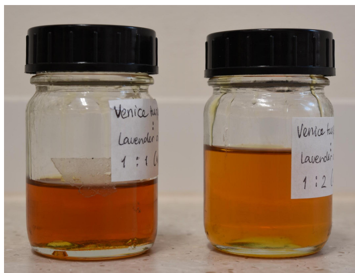
fig. 9 Two varnishes prepared of Venice turpentine and spike lavender oil, mixed in different ratios. Note the homogeneous state of the liquid, which means the resin has completely dissolved. (Photograph: S.Wouda)
