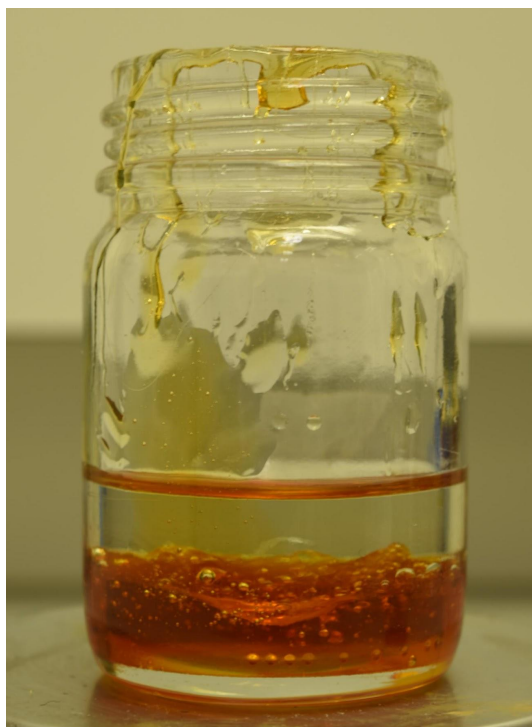
fig. 8 Venice turpentine and spike lavender oil (ratio 1:1), just after the oil was added to the resin. Note the stickiness of the resin. (Photograph: S.Wouda)
