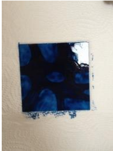
Figure 14 Quick and thin application of paint on whole surface using a brush
