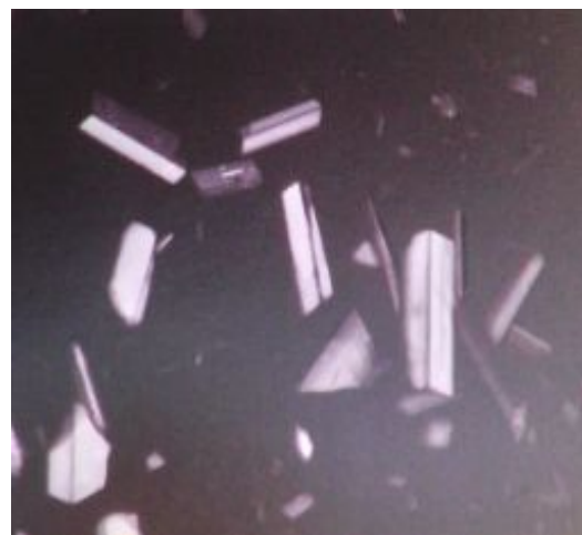
Figure 9. The smooth crystal surface of calcium sulfate particles enlarged 100x. This example shows gypsum particles, one of the several closely linked forms of calcium sulfate.
