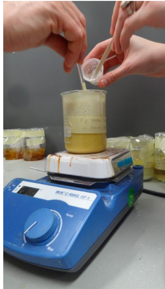
Figure 2. During the gradual addition of the chalk a bright yellow and opaque precipitate forms at the bottom of the beaker. This is the calcium sulfate to which the color of the dyestuff is attached by the mordanting function of the alum
