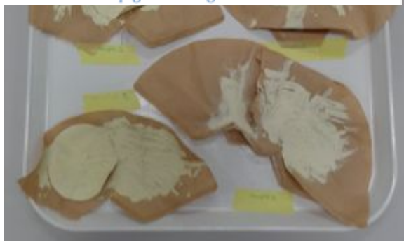
Figure 7. Four pigment samples made using the same amount of alum and dyestuff. The amount of chalk added to the sample in the right bottom corner was doubled as to the other three samples. It is obvious that the color of this pigment is lighter and less intense.
