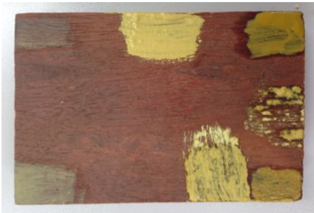
Figure 10. A piece of wood covered with the different paint samples. The yellow paint at the center of the top edge is mixed with egg white. This results in a bright and opaque yellow paint. The samples applied to the right top corner and right bottom corner are made with the same pigment as the pigment in egg white, but are here mixed with cold-pressed linseed oil. This results in a less bright, darker (more saturated) and more translucent paint as expected.
