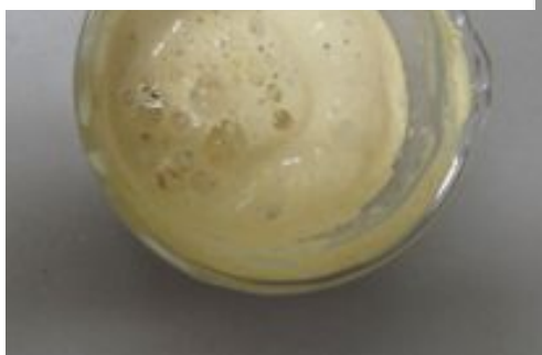
Figure 6. When the acidic conditions are neutralized by the addition of enough chalk, the formation of carbonic acid stops. The bubbles will become larger, the foam layer starts to get thinner and, finally, dissolves.
