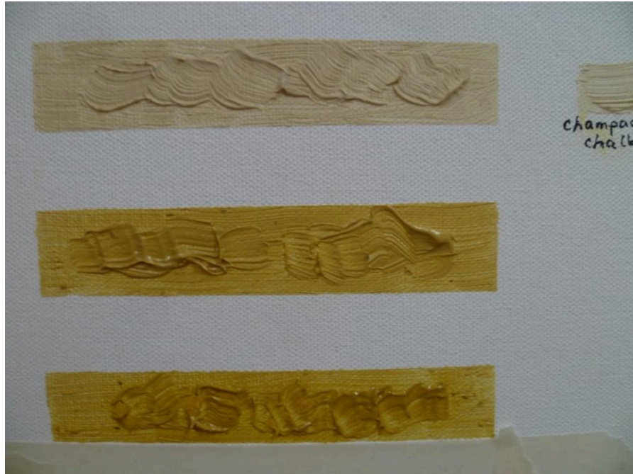
Fig. 1: Linseed oil paint samples made from weld lake pigments. In all cases, the pigment was extracted from weld by soaking the weld overnight and then boiling the weld for half an hour. The pigments were manufactured from recipe 5a from Natural Colorants for Dyeing and Lake Pigments: Practical Recipes and Their Historical Sources as a guide. From top: paint from pigment precipitated with only chalk, with reference of pure chalk mixed with oil to the right; paint from pigment precipitated with chalk and alum; paint from pigment precipitated with chalk and alum, with more concentrated weld juice. Note the lack of color in the pigment precipitated with only chalk, as the recipe for scudegrun on fol. 10r would seem to specify.
