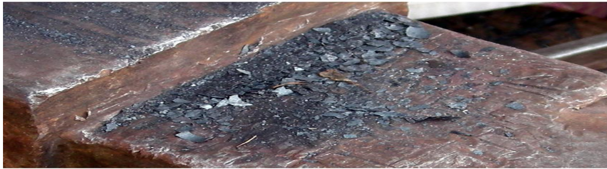
Fig. 1. Scales of iron as a side product from blacksmith work.
