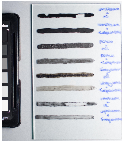
[Fig. 7] Reconstruction. “Scales black” applied with turpentine on glass in direct sun light (recto). Note the grey tone and the sparkle. A dark black was achieved with linseed oil resulting also in less sparkling.
