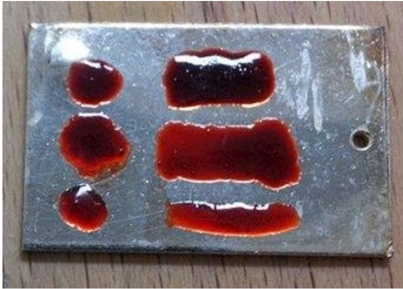
Fig. 12: Applying dissolved dragon's blood + mastic on silver. Beautiful translucent and uniform composition. Copyright: Picture by author.
