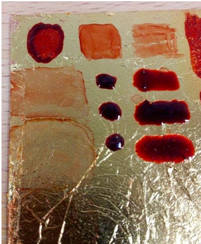
Fig. 13: Applying dissolved dragon's blood + mastic on gold. Beautiful translucent and uniform composition. Copyright: Picture by author.
