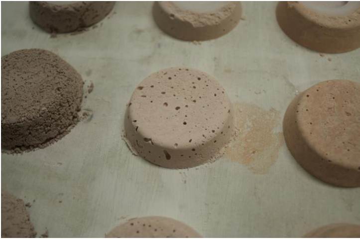
Fig. 19: The sand molds after drying
