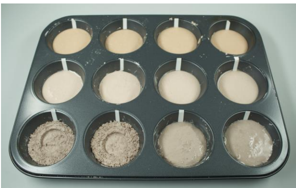
Fig. 18: The results of the sand- and liquid molds. From top to bottom: heavy spar, feldspar potassium and feldspar soda.
