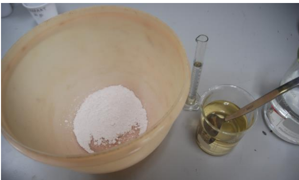
Fig. 3: Preparing the balls Fig. 4: Mixing the powder with the moisture, in this photo heavy spar.
