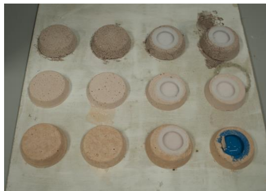
Fig. 16: The reaction of calcium oxide with water formed slaked lime.
