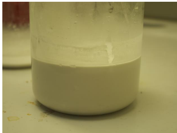
Fig. 16: The reaction of calcium oxide with water formed slaked lime.
