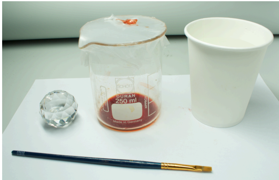
Fig. 11: The materials used for applying the dragon's blood au-bain-marie (hot water in the left cup) on a crystal.
