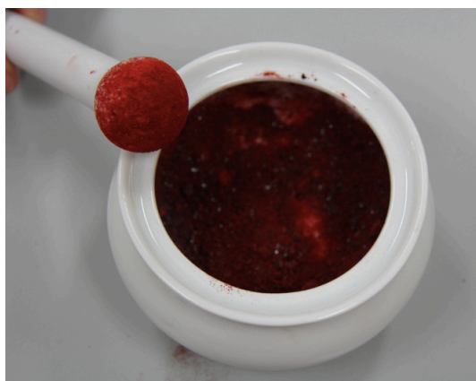
Fig. 3: Crushing the dragon's blood in a mortar.
