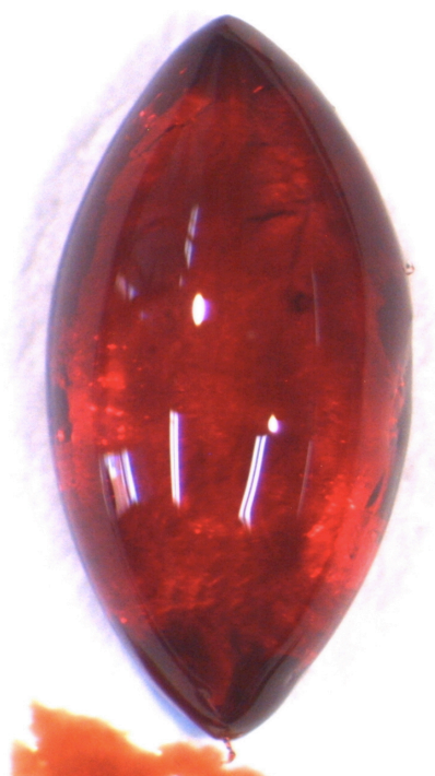
Fig. 10: Ruby colored with the dragon's blood substance (microscopic image with x2.5 magnification).
