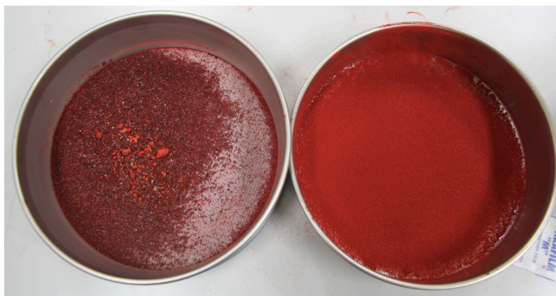
Fig. 4: The sieved dragon's blood powder on the right, the coarse powder and impurities on the left.
