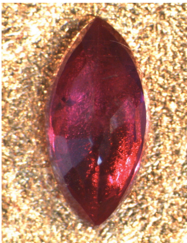
Fig. 9: Ruby placed on gold leaf which is colored by a thin solution of dragon's blood solved in ethanol (microscopic image with x2.5 magnification).
