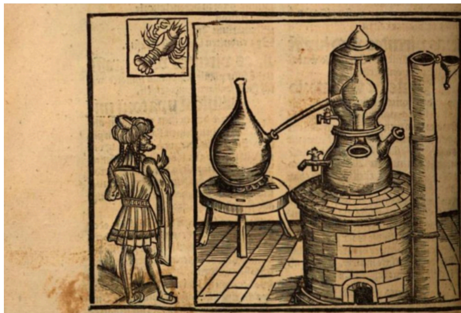
Fig. 2. Moor's Head Still, Brunshwyg, 1512 (GoogleBooks, accessed March 19th, 2016). This still is very advanced. The image shows the inside of the 'head', where the condensed material is collected and cooled by the vessel around this. The cucurbit can be filled without removing the top.
