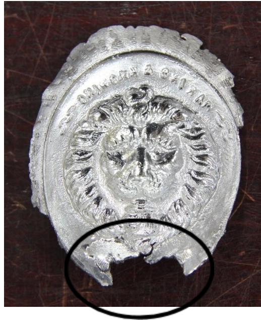
Fig. 11. Result of casting tin on brass, trial 1. Reverse
