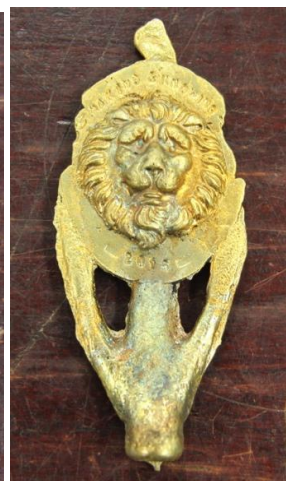
Fig. 40. Result of casting a new medal in brass, trial 5.
