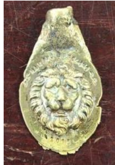
Fig. 18. Casting a brass medal, trial 3.
