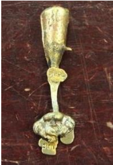
Fig. 16. Casting a brass medal, trial 1.
