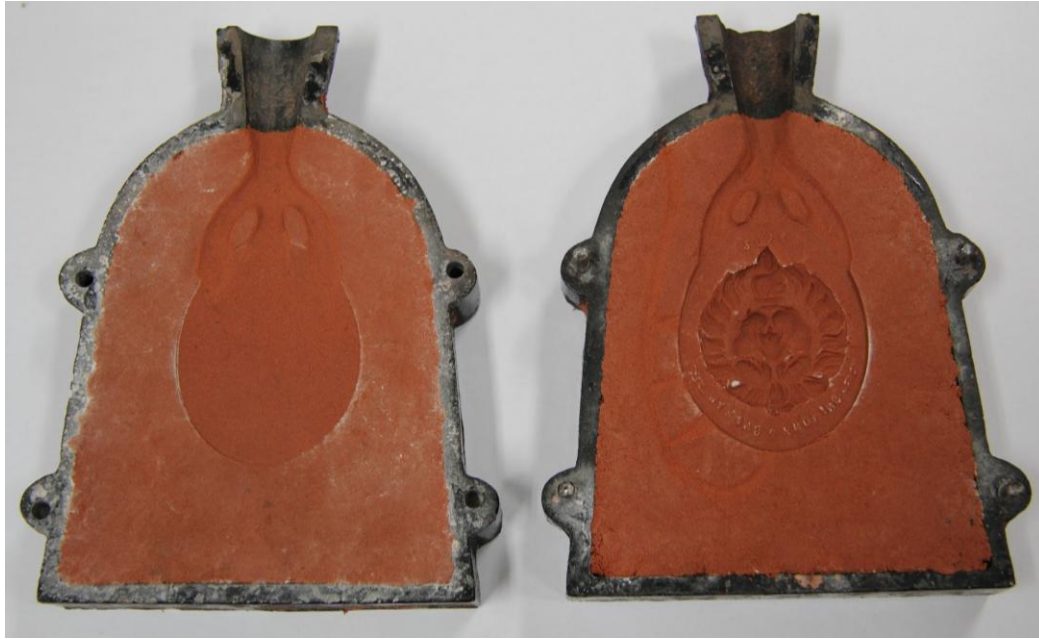
Fig. 63. Mould made for one of the bronze medal castings, using a sprue as was drawn by the author of the manuscript on folio 86v, 91v.
