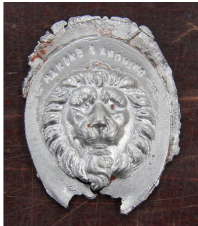
Fig. 49. Result of casting tin on tin, trial 1. Cast loosened from the original with the loss of a piece at the side of the sprue.
