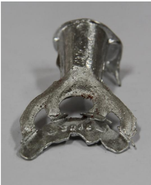
Fig. 57. Only a small part of the medal was cast.
