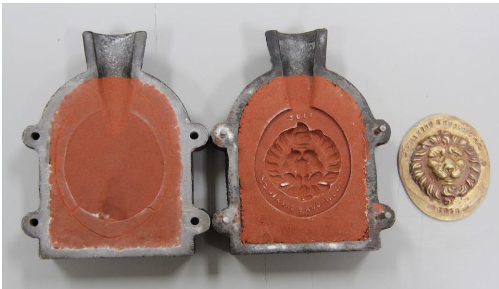
Fig. 62 The mould for one of the bronze cast medal where one big sprue was used.
