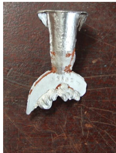
Fig. 51. Result of casting tin on tin, trial 2.
