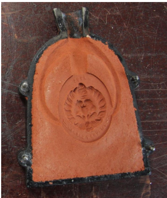
Fig. 37. Big casting flask with the mould of casting a new medal in brass, trial 5.
