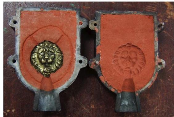
Fig. 25. Result of the mould, trial 4. Including sprues and vent-holes.
