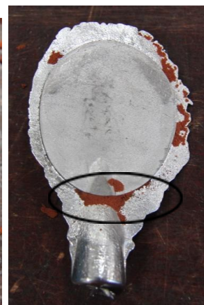
Fig. 47. Result of casting tin on tin, trial 1. Reverse. The circle indicates where the two medals got stuck.
