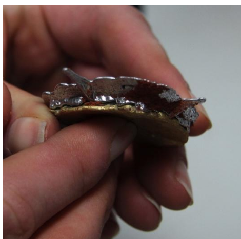
Fig. 27. Result of casting tin on brass, trial 1. Still stuck together.
