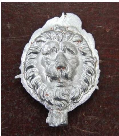
Fig. 6. Result of casting tin on brass, trial 4. Obverse.
