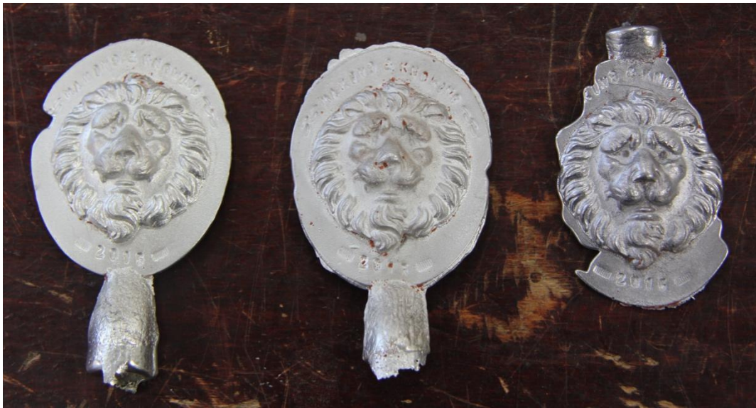
Fig. 44. Results of casting a new tin medal, trial 2, 3 and 4; counting from left to right.
