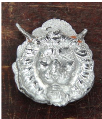
Fig. 2. Result of casting tin on brass, trial 1. Reverse.
