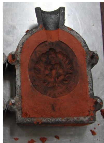
Fig. 38. Small casting flask with mould for casting tin on tin, trial 1.
