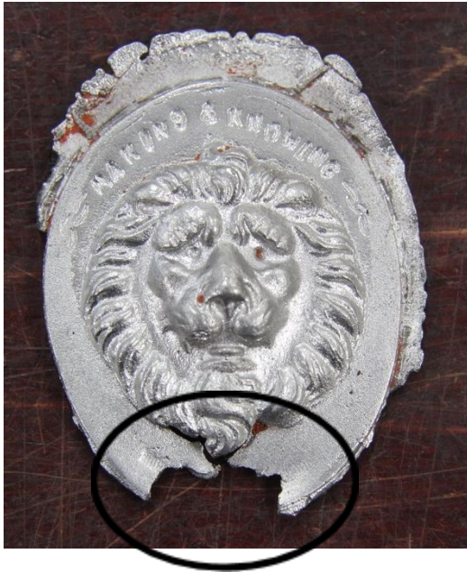
Fig. 10 Result of casting tin on brass, trial 1. Obverse. In the image the oval indicates where the incuse-reverse cast medal was stuck to the original
