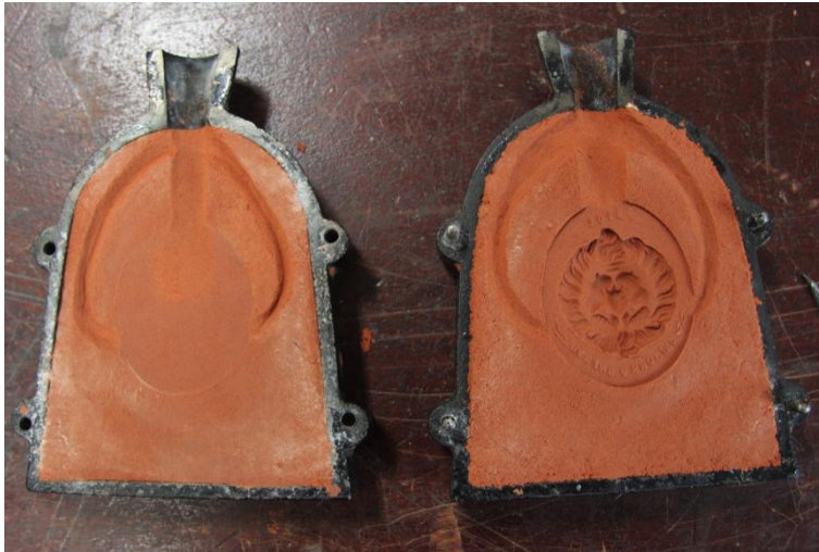
Fig. 41. Mould for casting a new medal in brass, trial 6. Forked sprue, pockets at the bottom were added later.
