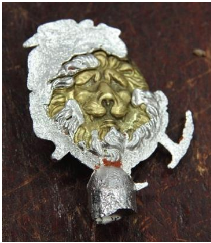
Fig. 5. Result of casting tin on brass, trial 3. Obverse.
