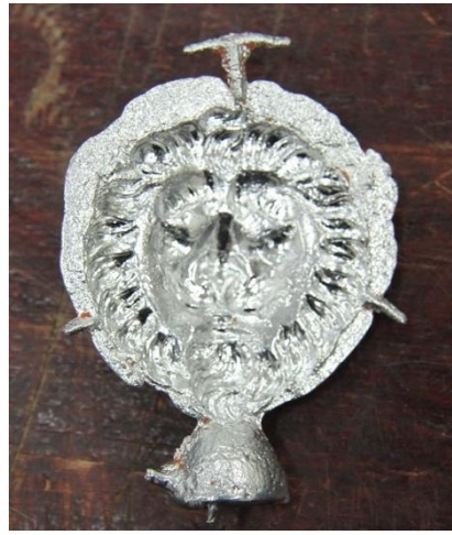
Fig. 9. Result of casting tin on brass, trial 5. Reverse.
