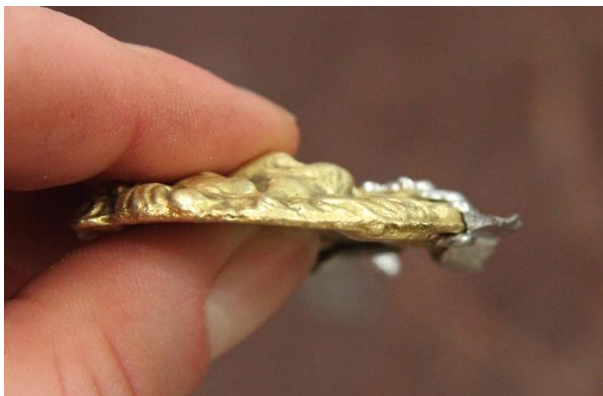
Fig. 30. Casting tin on brass, trial 3. Still stuck together, seen from the side.
