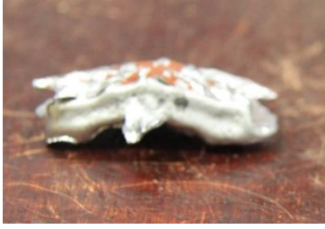
Fig. 29. Casting tin on brass, seen from the side.
