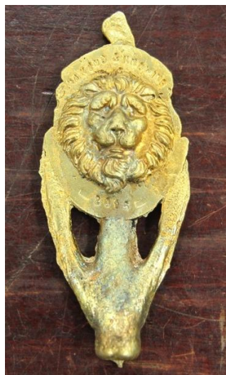
Fig. 17. Casting a brass medal, trial 2.
