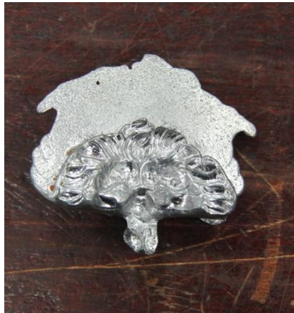
Fig. 4. Result of casting tin on brass, trial 2. Reverse.
