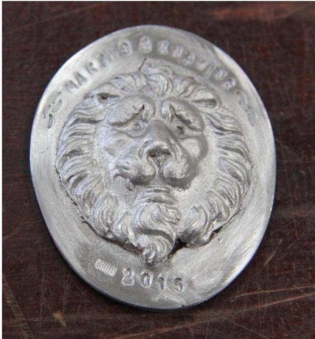
Fig. 43. Result of casting a new medal in tin, trial 1.
