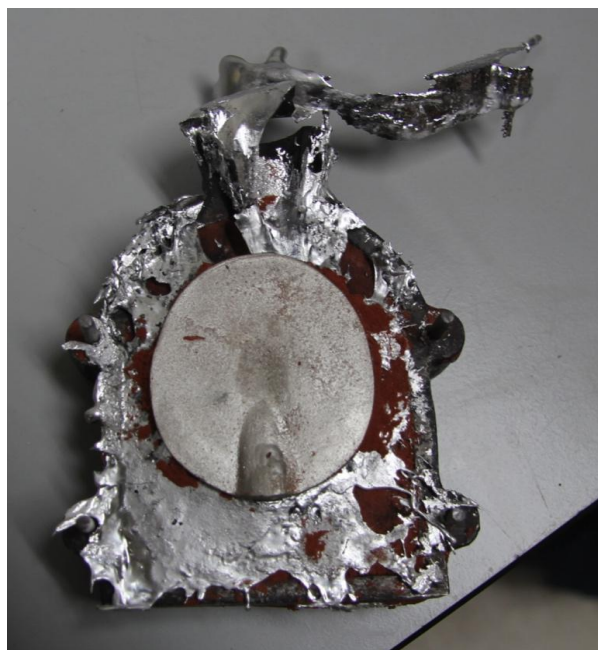
Fig. 53. Result of casting tin on tin, trial 4. Seen from the backside. still in the mould.
