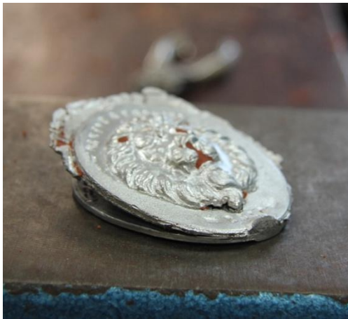
Fig. 48. Result of casting tin on tin trial 1. Original still attached at the side of the sprue, but loosened on the other side.
