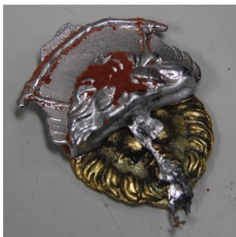
Fig. 28. Result of casting tin on brass, trial 2. Still stuck together.
