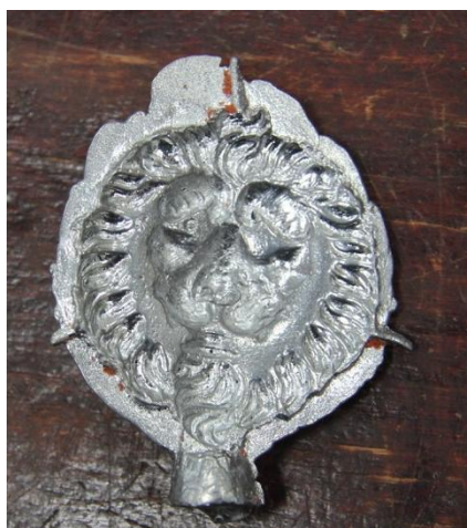
Fig. 7. Result of casting tin on brass, trial 4. Reverse.
