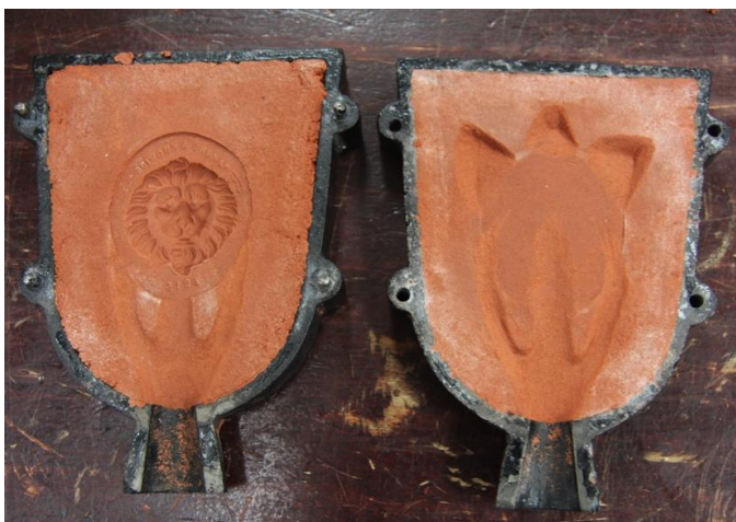
Fig. 39. Mould for casting a new medal in brass, trial 5. Forked sprue and pockets at the bottom.
