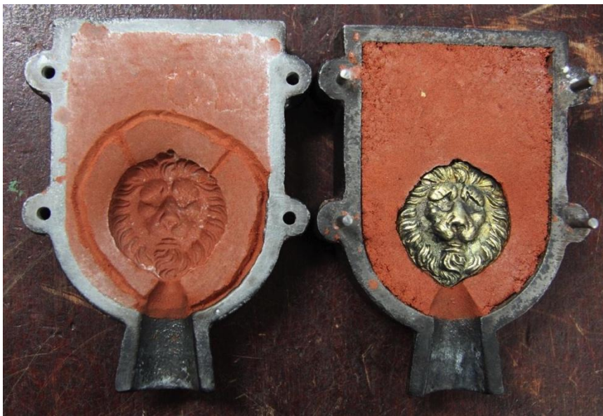
Fig. 26. Result of making a mould, trial 5. Including the sprue and vent-holes.
