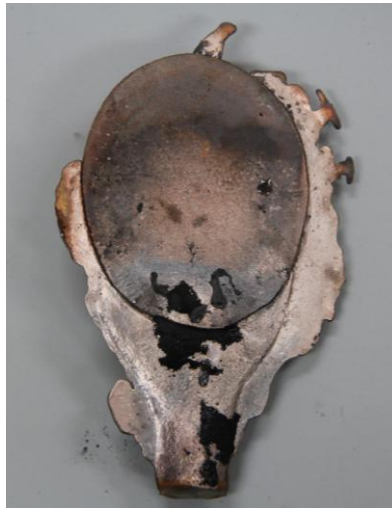
Fig. 66. Reverse of the bronze on bronze cast medal with original medal still attached.
