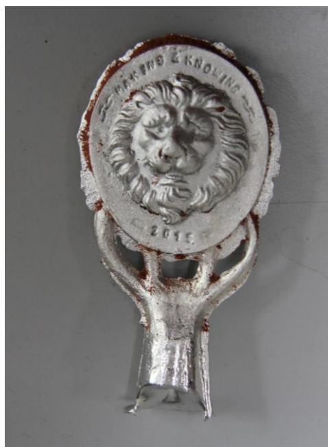
Fig. 60. The obverse of the cast medal. Fairly good detail obtained.
