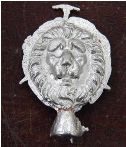
Fig. 8. Result of casting tin on brass, trial 5. Obverse.
