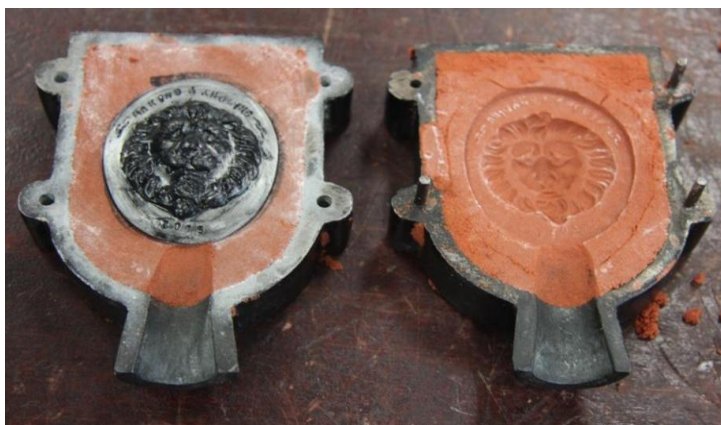
Fig. 46. Mould for casting tin on tin, trial 1.
