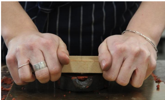
Fig. 24. Pressing the lion's head down with a piece of wood.
