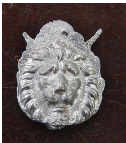
Fig. 1. Result of casting tin on brass, trial 1. Obverse.
