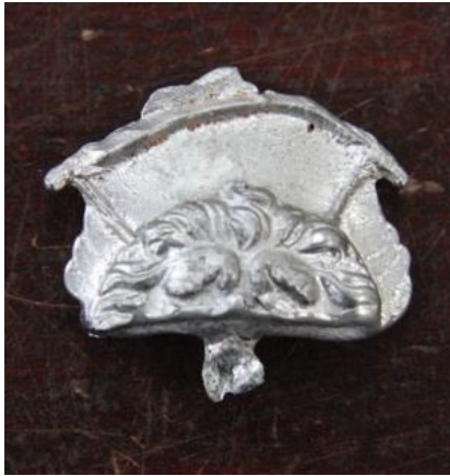
Fig. 3. Result of casting tin on brass, trial 2. Obverse.
