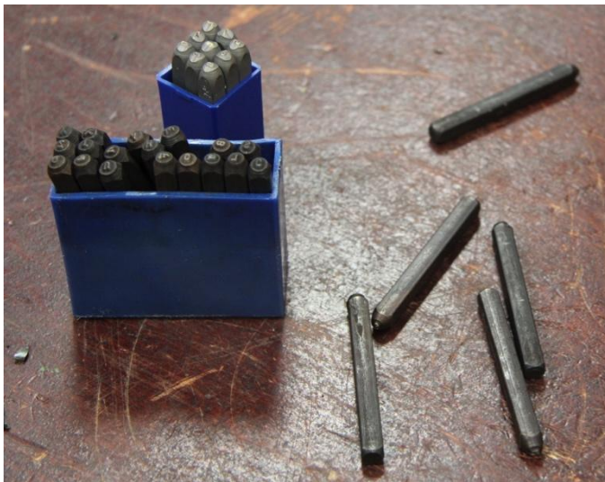
Fig. 32. Punches used for applying letters and details onto the medal.
