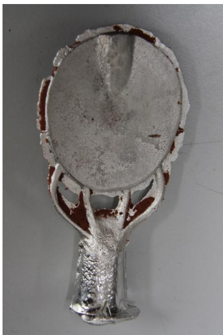
Fig. 59. Tin on tin cast. Both clammed together.
