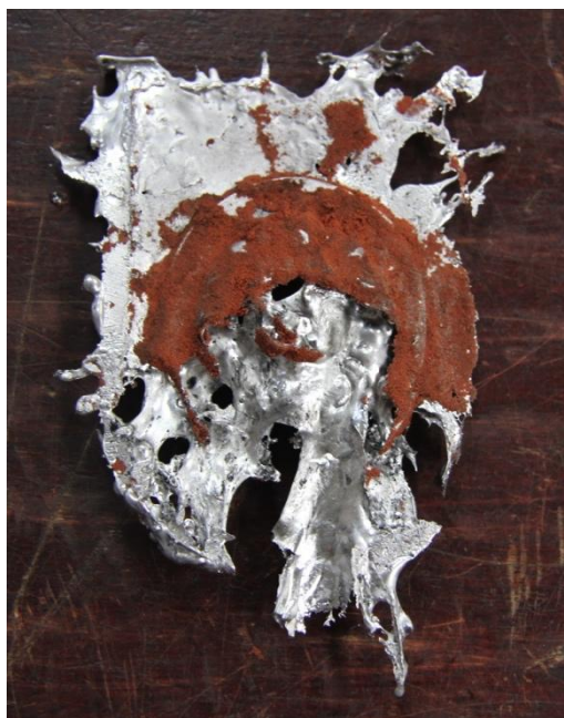
Fig. 54. Result of casting tin on tin, trial 4. Obverse.
