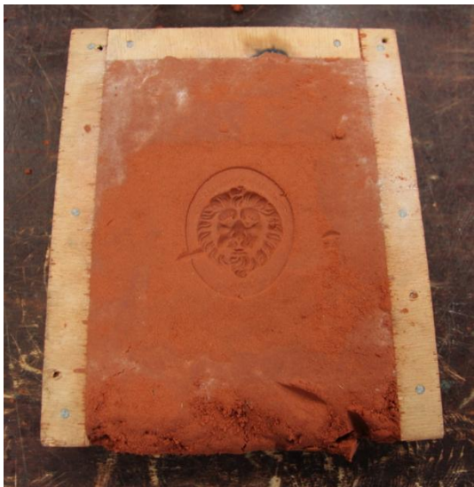
Fig. 35. Wooden box mould in which it was tried to make a mould.
