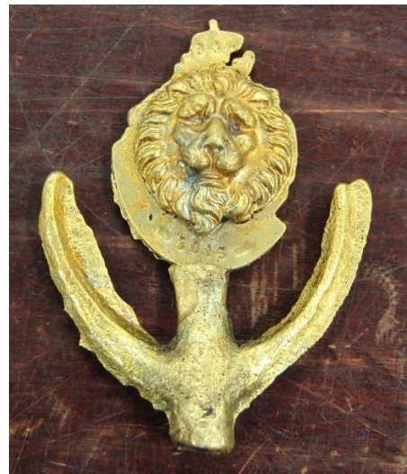
Fig. 18. Casting a brass medal, trial 3.
