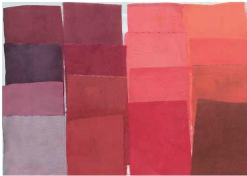
20. Samples of silk cloth dyed with cochineal, showing the many different hues that can be achieved by adding mordants and other modifiers to the dyebath
